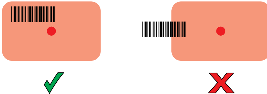
Figure 79 DS3608/DS3678 Pick List Mode with Multiple Barcodes in Aiming Pattern
