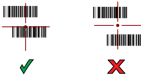
Figure 73 RS507/RS507X Pick List Mode with Multiple Barcodes in Aiming Pattern
