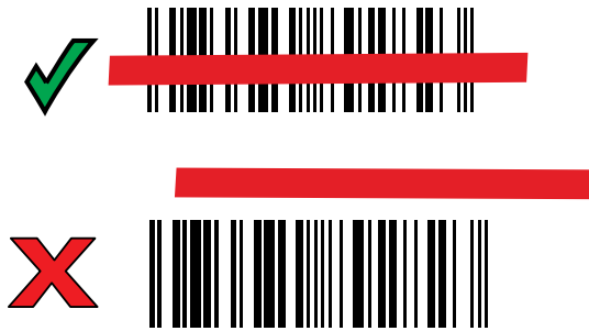
Figure 81 DS2278 Aiming Pattern
