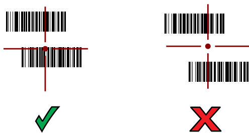
Figure 76 RS6000 Pick List Mode with Multiple Barcodes in Aiming Pattern
