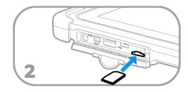
**Note:** Always power off the tablet before attempting to install or remove a card.
