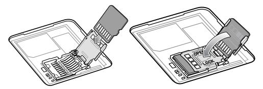
5. Close the microSD card holder and lock into position.
