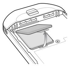
2. Slide the microSD card holder to the unlock position.
