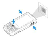
4. Touch **Scan** on the screen or press and hold any Scan button. Center the aiming beam over the barcode.
