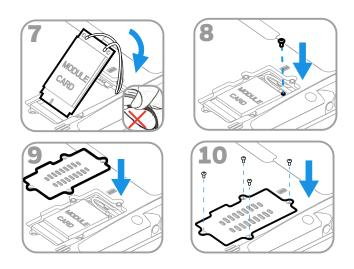
**Note:** Always power off the tablet before attempting to install or remove a card.
