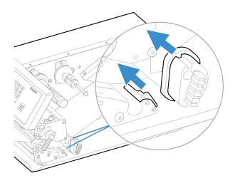
13. Close the front door and media cover. Make sure that the media runs through the slot in the front door.
