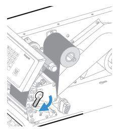
8. Press the cardboard core at the front end of the ribbon onto the rewind hub. During printing, the rewind hub rotates counter-clockwise.
