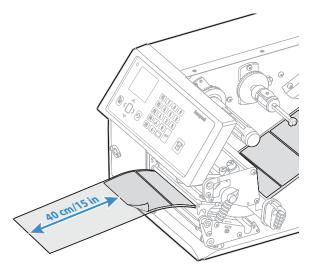
12. Route the liner around the tear bar and back under the print unit.
