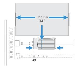
6. Press the ribbon roll onto the ribbon supply bobbin and route the ribbon through the print unit. Pull out 20 cm (8 in) of ribbon.
