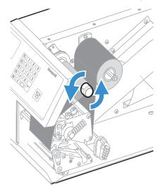
11. Turn the printhead lift lever clockwise to lower the printhead.
