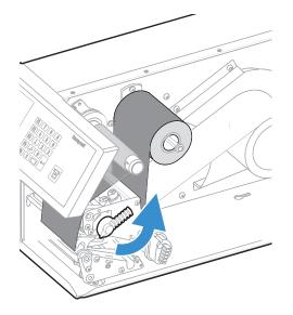
5. If necessary, remove the empty core from the media supply roll post.
