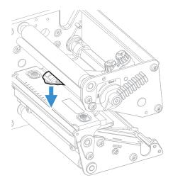
7. Disconnect the hooks of the printhead bracket from the shaft and pull out the printhead as far as the cables allow.
