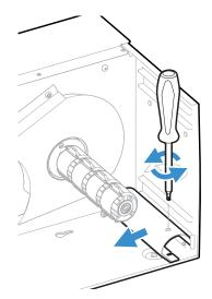
6. Remove the tear bar from the print unit and replace it with the guide plate.
