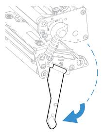
4. Raise the printhead by turning the printhead lift lever counter-clockwise.
