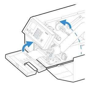
18. Press the **Print/Feed** button to advance the media and adjust the media feed.
