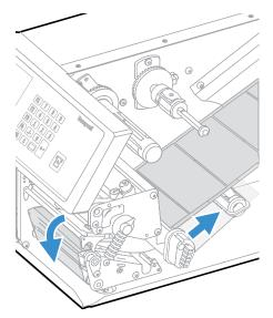
13. Secure the liner to the take-up hub with the red clip and rotate the hub until the media is pulled tight.
