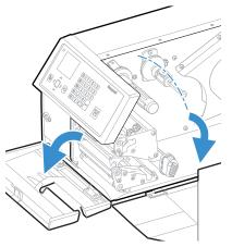
2. Pull the upper guide straight out and press the snap-lock, lift the edge of the lower guide, and pull the lower guide straight out.
