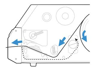
10. Turn the printhead lift lever clockwise to lower the printhead.
