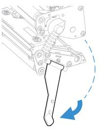
4. Turn the printhead lift lever counter-clockwise to raise the printhead.
