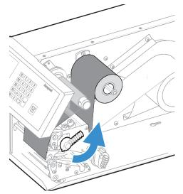
5. Pull out the red clip on the liner take-up hub and dispose of any wound-up liner.
