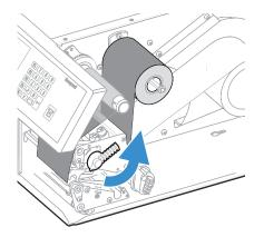
5. Remove any empty core from the media supply hub.
