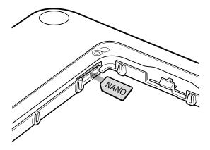
Figure 11 Inserting the nano SIM Card - 10.1"
