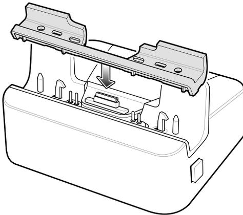
2. Press the insert down until it seats flush in the cradle.
