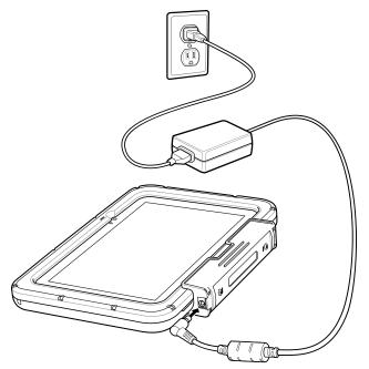
Charge batteries in ambient temperatures from 0°C to +60°C (32°F to 140°F) as reported by the battery. Charging is intelligently controlled by the charger. To accomplish this, for small periods of time, the charger alternately enables and disables battery charging to keep the battery at acceptable temperatures.
