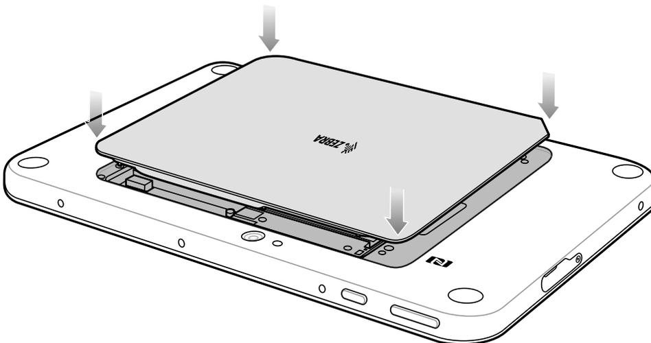
3. Carefully press down around the edge of the cover. Make sure that the cover is seated properly.
