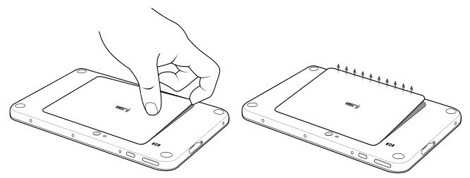
4. On the 8.4" version, push the two locking tabs up, then pull up on the tab to remove battery.On the 10.1" version, push the two locking tabs up (1), then, using index fingers, lift the battery up (2).
