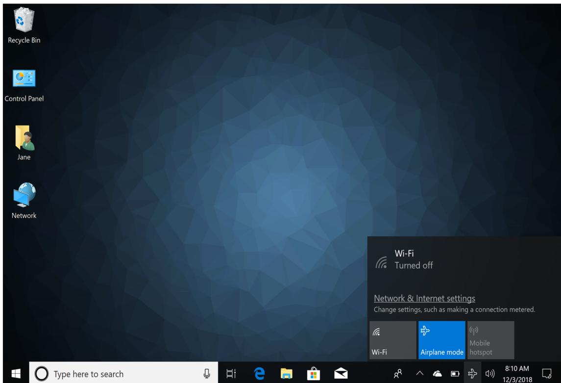
To turn on radios in Airplane Mode (without turning on WAN):
