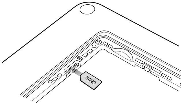
2. Push the SIM card in and ensure that it locks into place.
