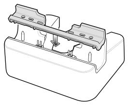
2. Press the insert down until it seats flush in the cradle.
