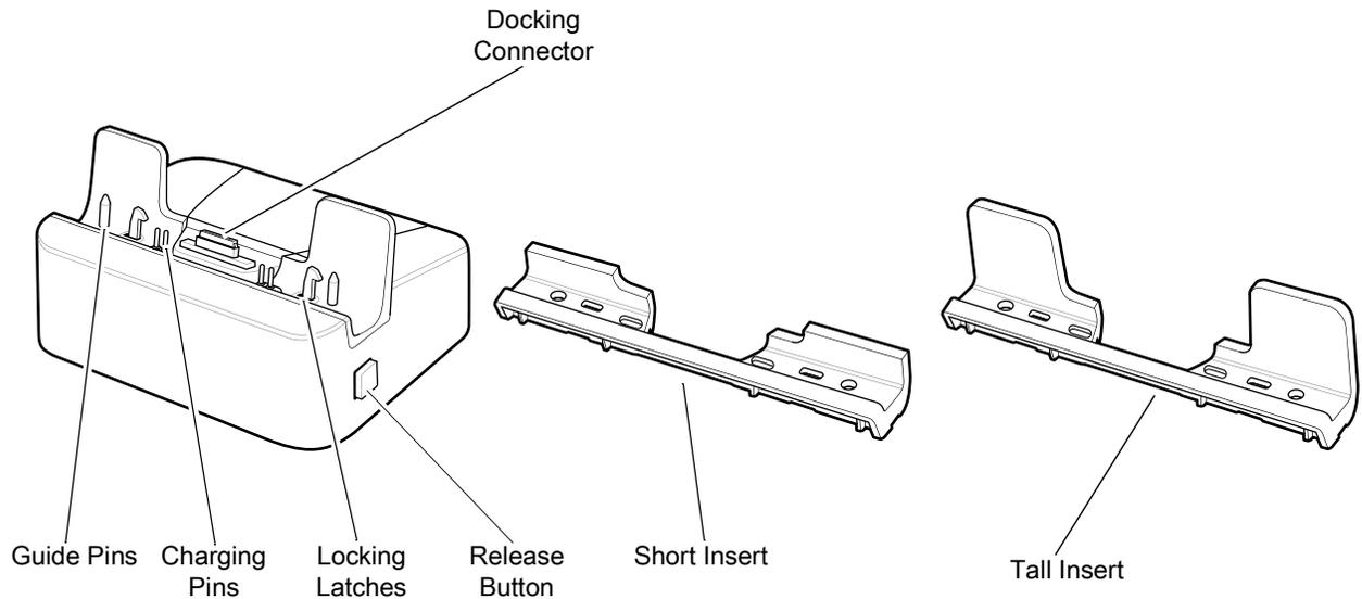
**Figure 66** Communication and Charging Cradle - Rear View
