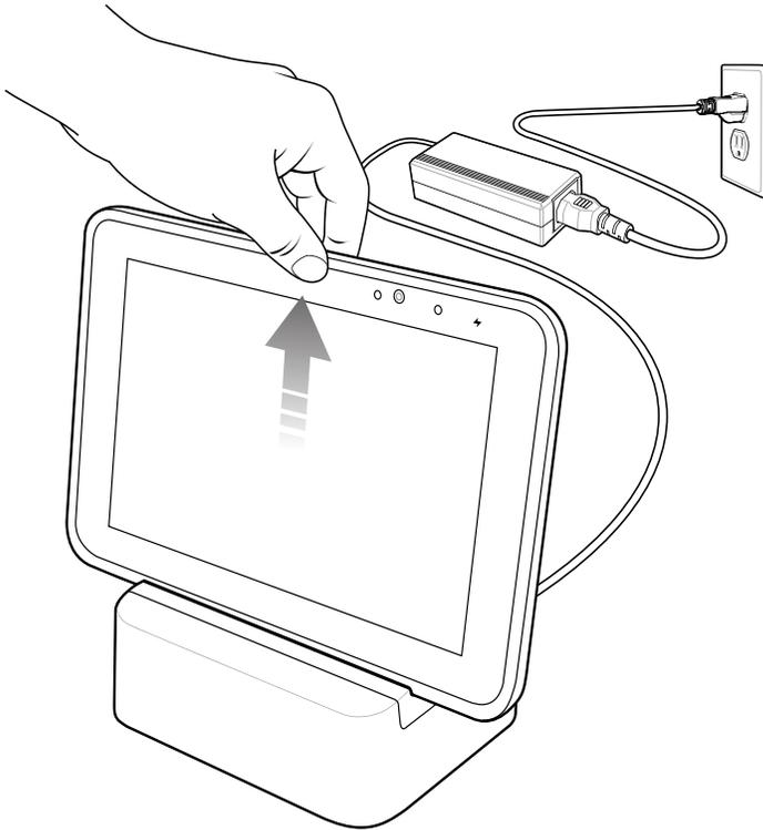
Charge batteries in ambient temperatures from 0°C to +60°C (32°F to 140°F) as reported by the battery. Charging is intelligently controlled by the charger. To accomplish this, for small periods of time, the charger alternately enables and disables battery charging to keep the battery at acceptable temperatures.
