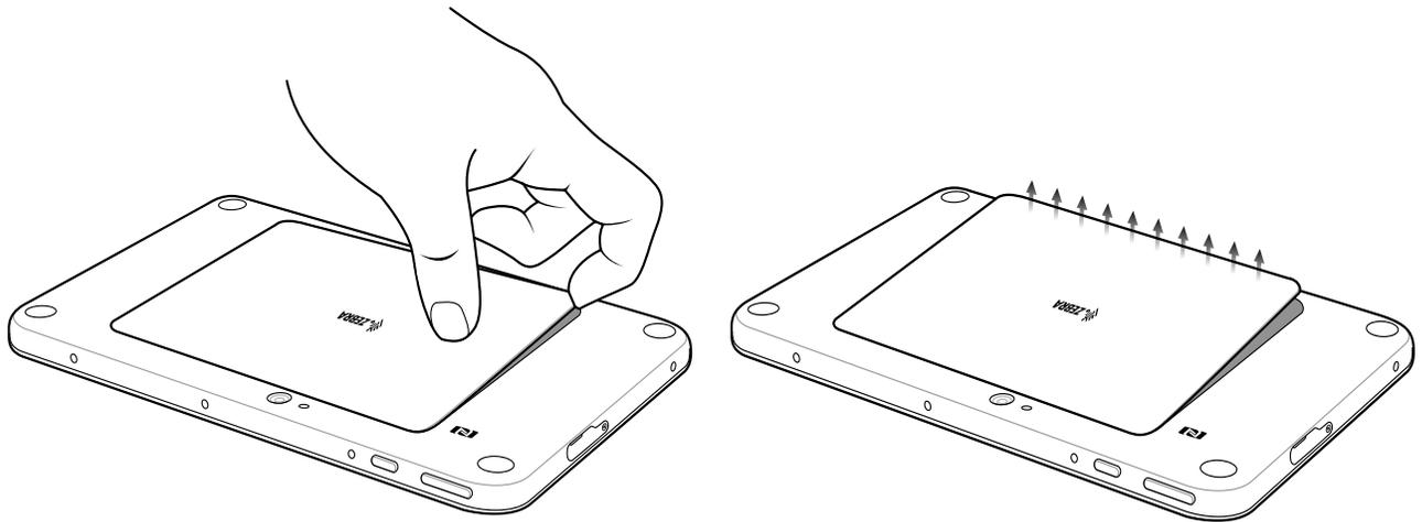
4. On the 8.4" version, push the two locking tabs up, then pull up on the tab to remove battery.
