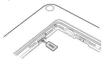
2. Push the SIM card in and ensure that it locks into place.
