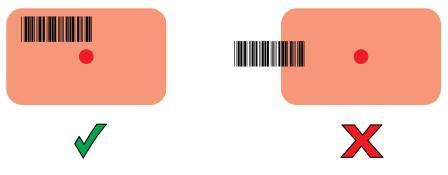
Figure 49 DS3608/DS3678 Pick List Mode with Multiple Barcodes in Aiming Pattern
