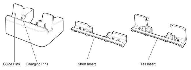
Figure 61 Charge Only Cradle - Rear View
