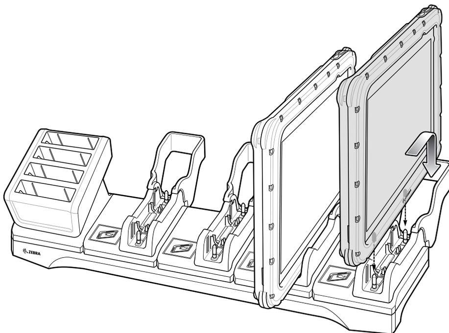
3. Place the device down into the slot with display facing away from Battery Charger.
