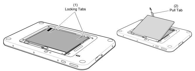
Figure 8 Removing the Battery - 10.1"
