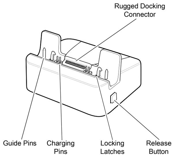
**Figure 71** Rugged Communication and Charging Cradle - Rear View
