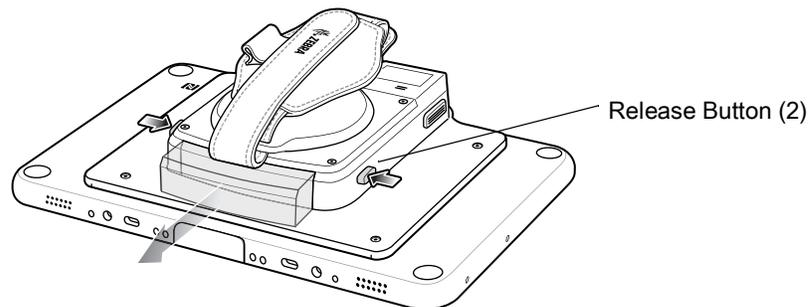
3. Remove dummy battery insert.
