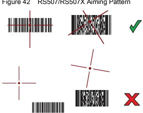
Figure 42 RS507/RS507X Aiming Pattern
