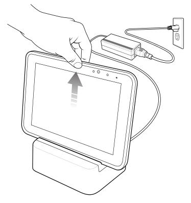
Charge batteries in ambient temperatures from 0°C to +60°C (32°F to 140°F) as reported by the battery. Charging is intelligently controlled by the charger. To accomplish this, for small periods of time, the charger alternately enables and disables battery charging to keep the battery at acceptable temperatures.
