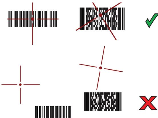
Figure 43 RS507/RS507X Pick List Mode with Multiple Barcodes in Aiming Pattern
