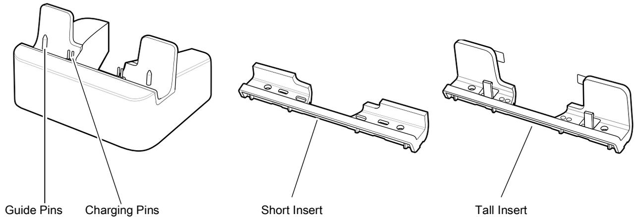
**Figure 61** Charge Only Cradle - Rear View
