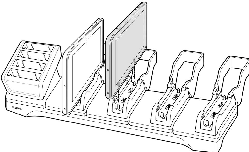
3. Place the device down into the slot with display facing away from Battery Charger.
