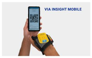
Open the app symbol "Insight Mobile" on the mobile device and scan the Pairing Barcode. To download the app and configure the device, register at <a href="https://www.datalogic.com/handscanner/config">https://www.datalogic.com/handscanner/config</a>.
