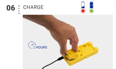
The pins face down. Insert the HandScanner in the Datalogic Charging Station.
